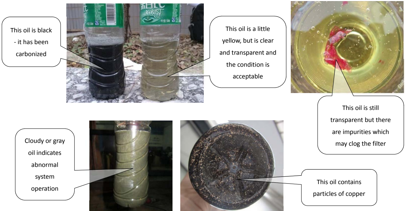
Figure 6-2.10: Inspecting compressor oil
