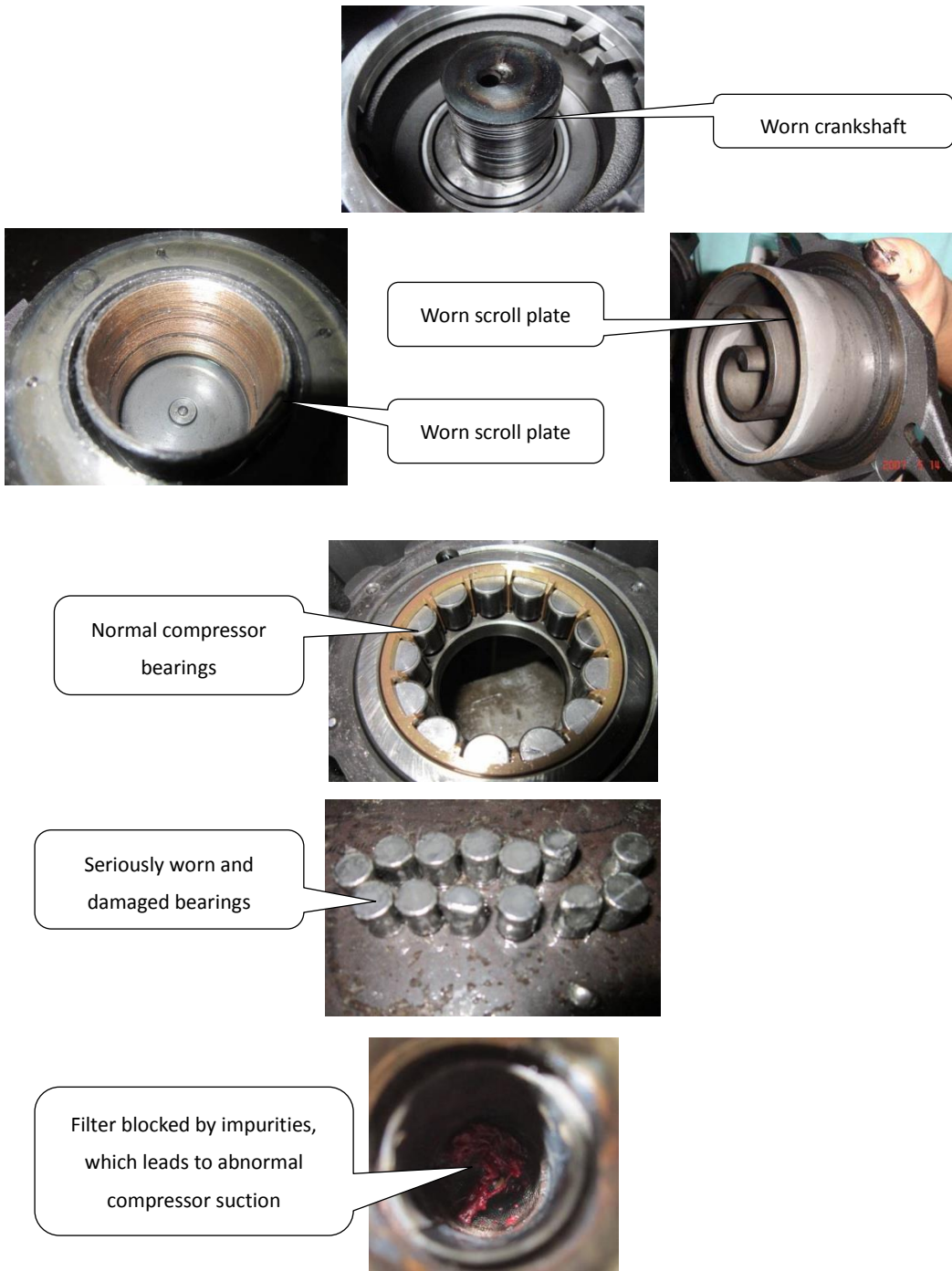
Figure 6-2.11: Effects of spoiled compressor oil
