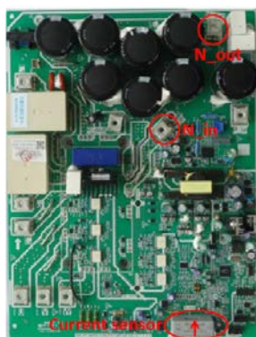
Figure 6-2.2: DC detection wire connection method
