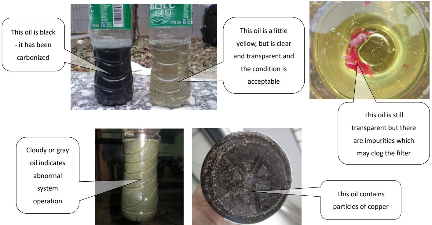
Figure 6-2.10: Inspecting compressor oil
