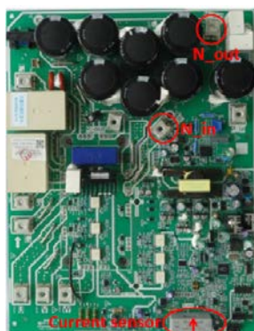
Figure 6-2.5: DC detection wire connection method
