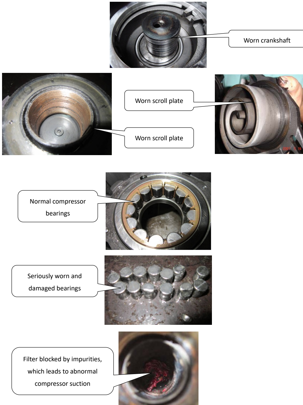
Figure 6-2.11: Effects of spoiled compressor oil
