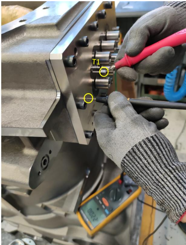
Figure 39 Electrical insulation terminal thermistor - earth
