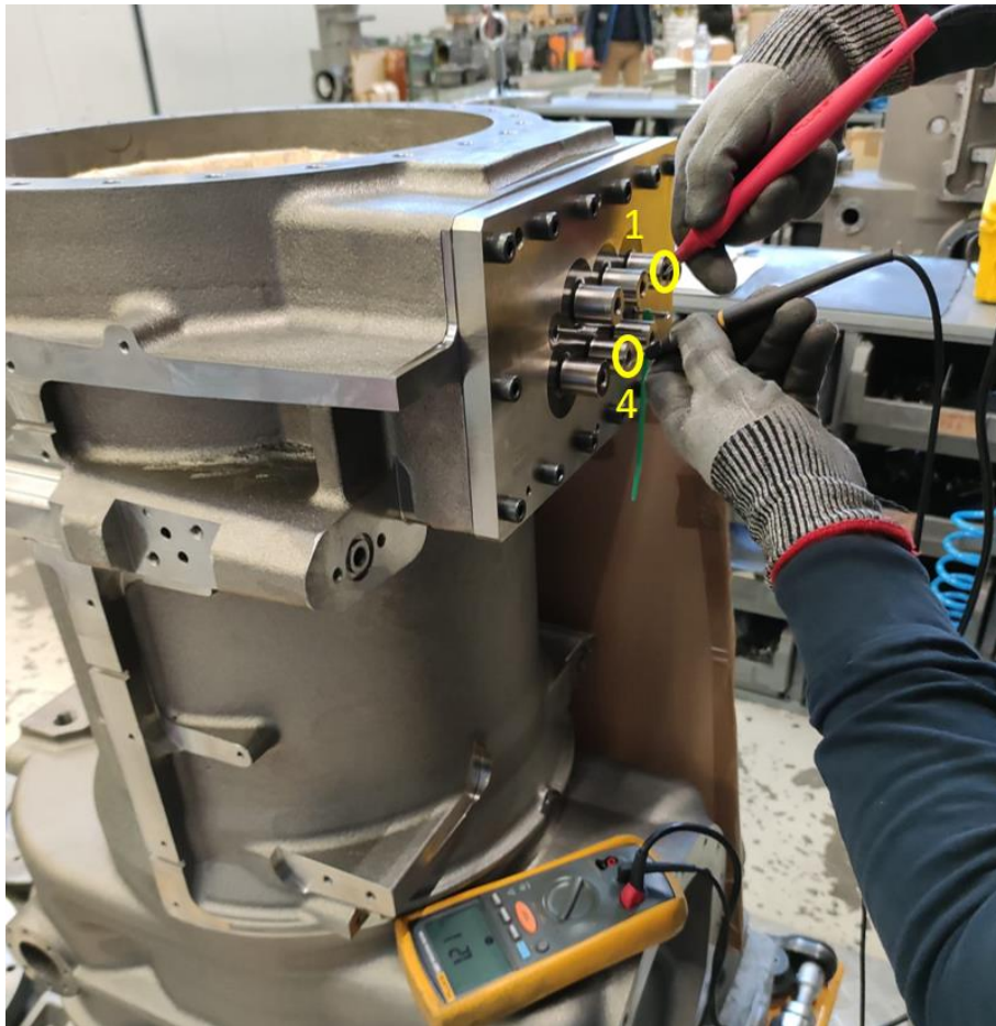
Figure 51 Motor phases electrical continuity
